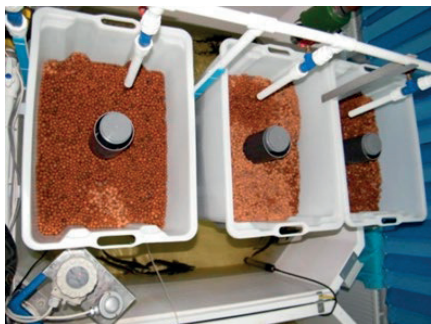
Figure 1: Control variant consist in aquaponic modules with no plants, only substrate - light expanded clay aggregate (LECA)
