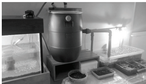
Figure 2. The aquaponic system
