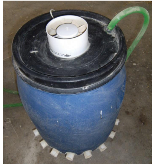
Figure 1. Designed ammonia trap system
