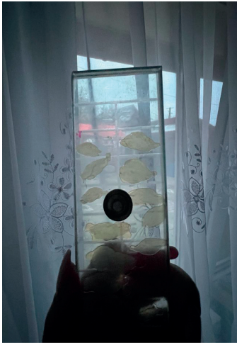
Figure 1. The arrangement of the meat samples between the blades for the trichinelloscopic examination
