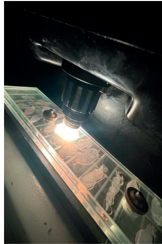
Figure 2. Placement under the microscope of slides with meat samples for the trichinelloscopic examination (Own source)
