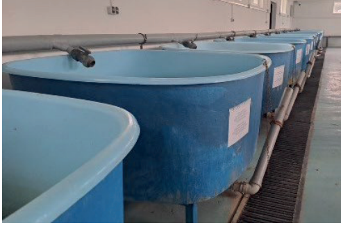
Figure 1. Evostype fiberglass tanks (original photo)
