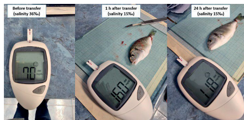
Figure 2. Blood glucose readings on gilthead seabream before, one hour and 24 hours after transfer from 36‰ to 15‰ salinity ( Original photos )
