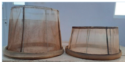
Figure 3. The new filter- on the left side; the old filter - on the right side (original)
